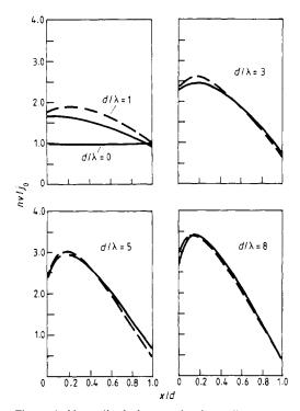
Figure 1. Normalised electron density  $nv/j_0$  versus normalised distance x/d for various normalised gas pressures  $d/\lambda$  for the case of zero electric field (solid line). The dashed line represents the numerical results of Bartels and Noak (1930).
