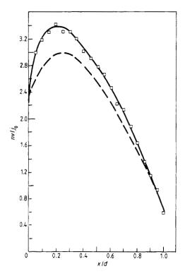
Figure 4. Normalised electron density  $nv/j_0$  versus normalised distance for r = 1. The full and dashed curves correspond to the Monte-Carlo and analytical methods respectively.
