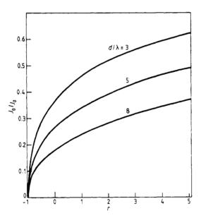
Figure 3. Normalised current to the anode  $J_0/j_0$  versus normalised electric field r for various normalised gas pressures.
