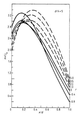
Figure 2. Normalised electron density  $nv/j_0$  versus normalised distance x/d for various normalised electric field  $r = 2eEd/mv_0^2$ . All curves correspond to the case of  $d/\lambda = 5$ .
